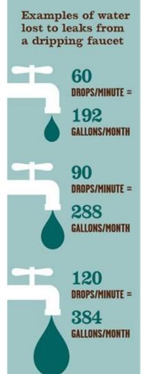
EPA WaterSense program is sponsoring "Fix a Leak Week" March 16-22 to remind Americans to check their plumbing fixtures and irrigation systems for leaks. The WaterSense website <a href="www.epa.gov/watersense">www.epa.gov/watersense</a> offers useful tips and videos about leak identification and repair. Leak detection and repair inside the house is often very easy and simple and is a great first step toward creating a water efficient home.
